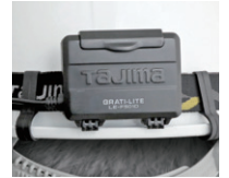
The external battery compartment
