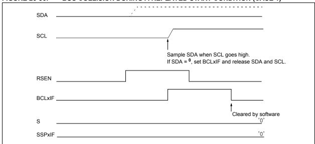
FIGURE 26-37: BUS COLLISION DURING REPEATED START CONDITION (CASE 2)
