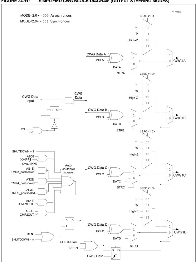
**FIGURE 24-11:** SIMPLIFIED CWG BLOCK DIAGRAM (OUTPUT STEERING MODES)
