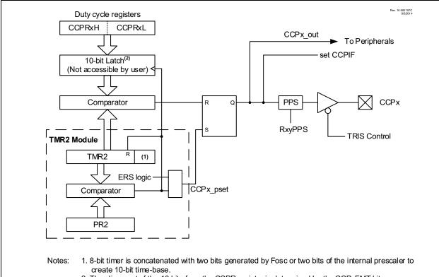
2. The alignment of the 10 bits from the CCPR register is determined by the CCPxFMT bit.
