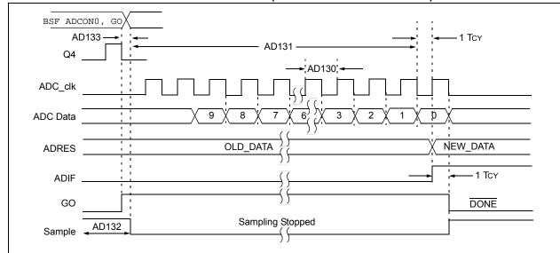
Note 1: If the ADC clock source is selected as ADCRC, a time of Tcy is added before the ADC clock starts. This allows the SLEEP instruction to be executed.
