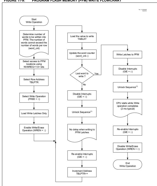
**FIGURE 11-9:** PROGRAM FLASH MEMORY (PFM) WRITE FLOWCHART
