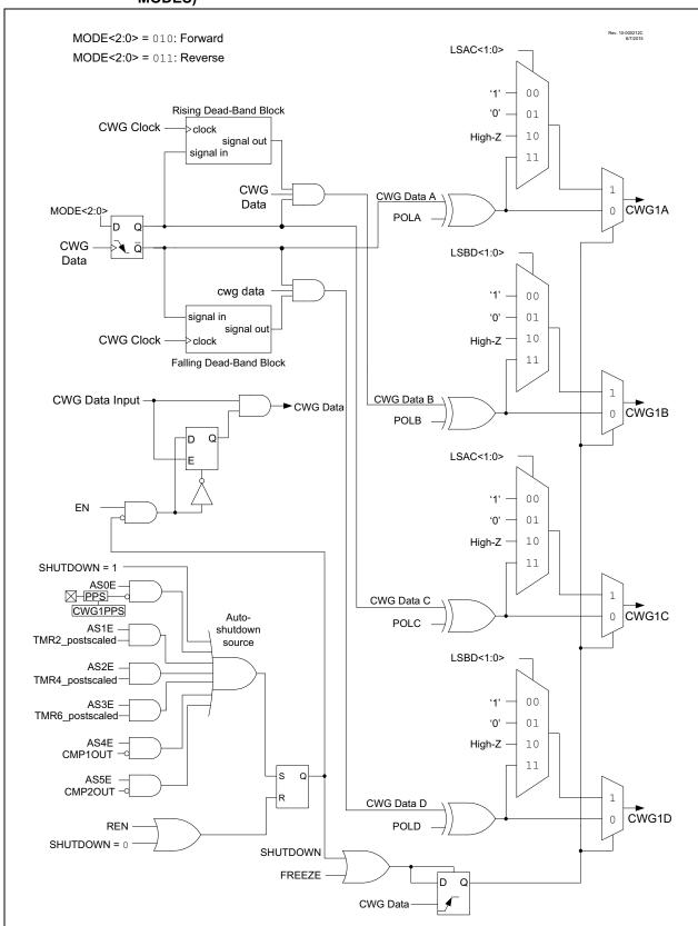
FIGURE 24-6: SIMPLIFIED CWG BLOCK DIAGRAM (FORWARD AND REVERSE FULL-BRIDGE MODES)
