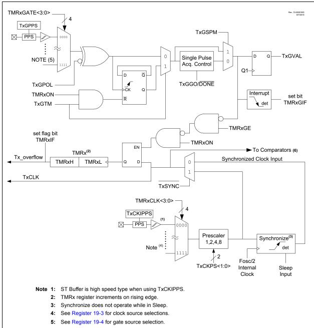
6: Synchronized comparator output should not be used in conjunction with synchronized input clock.
