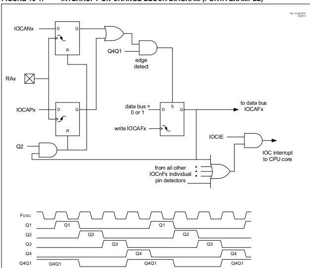
FIGURE 16-1: INTERRUPT-ON-CHANGE BLOCK DIAGRAM (PORTA EXAMPLE)
