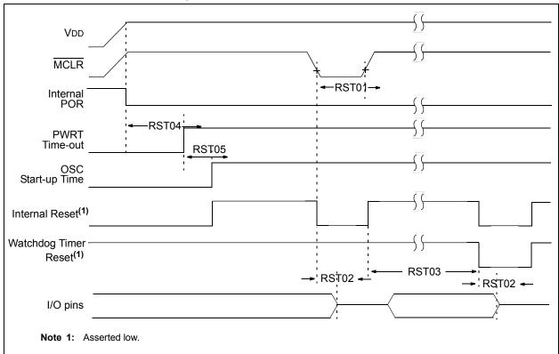
FIGURE 37-9: BROWN-OUT RESET TIMING AND CHARACTERISTICS
