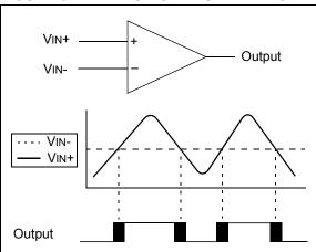
**Note:** The black areas of the output of the comparator represents the uncertainty due to input offsets and response time.
