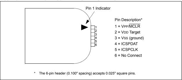
FIGURE 34-3: TYPICAL CONNECTION FOR ICSP™ PROGRAMMING
