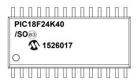
28-Lead SSOP (5.30 mm)
