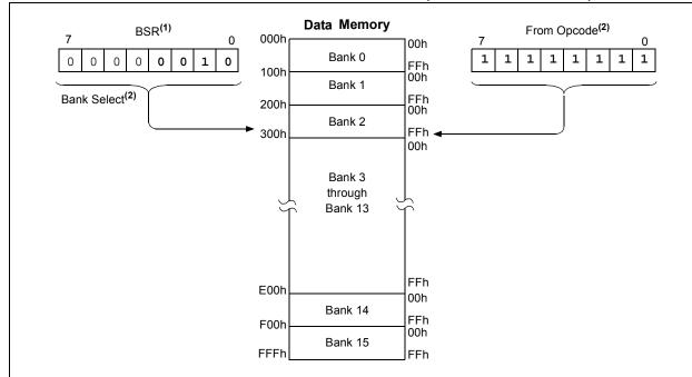
Note 1: The Access RAM bit of the instruction can be used to force an override of the selected bank (BSR<3:0>) to the registers of the Access Bank.
