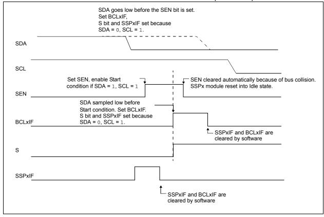
FIGURE 26-34: BUS COLLISION DURING START CONDITION (SCL = 0)
