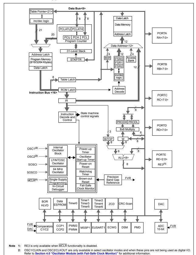
FIGURE 1-1: PIC18(L)F24/25K40 FAMILY BLOCK DIAGRAM
