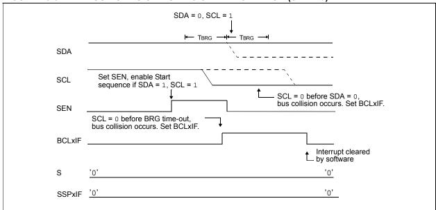
FIGURE 26-35: BRG RESET DUE TO SDA ARBITRATION DURING START CONDITION
