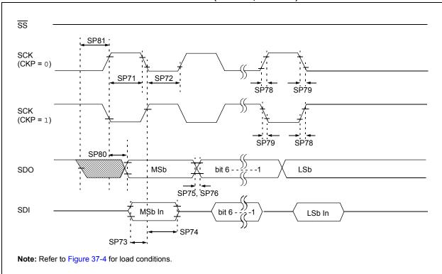
FIGURE 37-17: SPI MASTER MODE TIMING (CKE = 1, SMP = 1)
