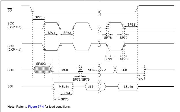
FIGURE 37-19: SPI SLAVE MODE TIMING (CKE = 1)
