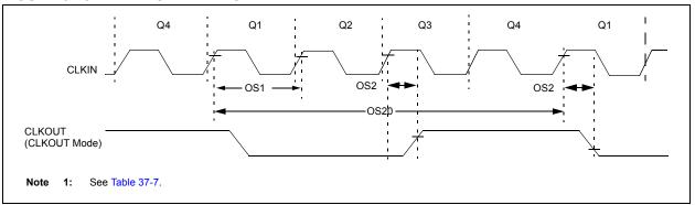
TABLE 37-7: EXTERNAL CLOCK/OSCILLATOR TIMING REQUIREMENTS
