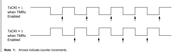
2: In Counter mode, a falling edge must be registered by the counter prior to the first incrementing rising edge of the clock.
