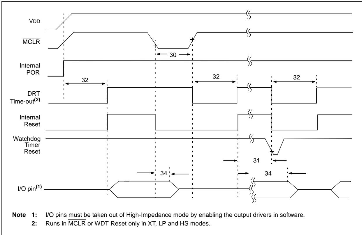
**Note 1:** I/O pins must be taken out of High-Impedance mode by enabling the output drivers in software.
