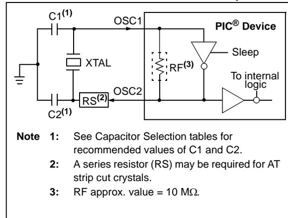
**FIGURE 8-2: EXTERNAL CLOCK INPUT OPERATION (HS, XT, LP OR EC OSC CONFIGURATION)**
