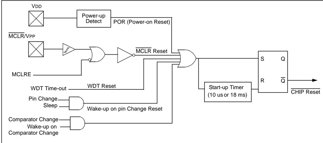
**FIGURE 8-8: TIME-OUT SEQUENCE ON POWER-UP ( $\overline{\text{MCLR}}$  PULLED LOW)**
