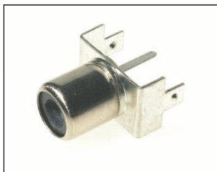
PHS-7A Vertical PCB mounting RCA Phono connector. Several different coloured inserts available. Nickel Silver or Gold plated finish. PHS-7A (FC68400)
