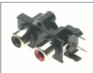
PHS-10B PCB mounting dual RCA Phono connector. Several different coloured inserts available. Nickel Silver or Gold plated finish. PHS-10B (Various)
