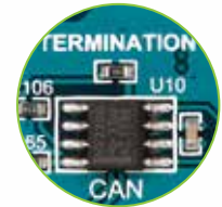
Figure 16-2: CAN transceiver with Node TERMINATION jumper
