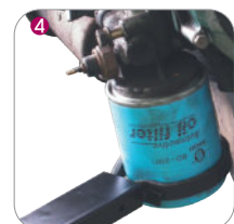
• Oil filter removal & assembly
