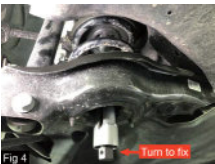
• Turn the hex nut on the main tool body lower end to fix all parts
