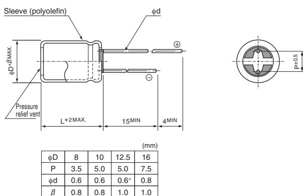
\* In case L &gt; 25 for the φ12.5 dia. unit, lead dia. φ d = 0.8mm.
