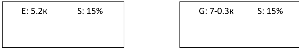
(«E: 5.2k» - rate of transmitting via Ethernet 5,2 kB/sec, «G: 7-0.3k» - the level of GSM signal is 70%, rate of transmitting via GSM GPRS is 0,3 kB/sec, «S: 15%» - Loading of RS-485 is 15%)
