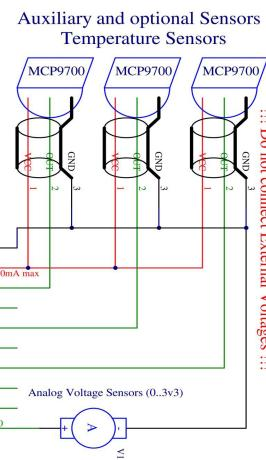
Shielded wires (2+shield) - shield connected to GND
