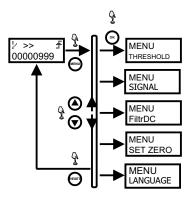
tTo select menu use buttons UP or DOWN. Pass to choosen menu is possible by pressing button OK. Return to main menu is make by pressing button RESET.
