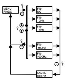
After you select a menu FiltrDC press OK. Then, using the UP and DOWN buttons to select the appropriate frequency filtering and approve it OK. Exit menu without saving changes is possible by pressing the RESET button. Set the menu item in FiltrDC doesn't mean exclusion of the internal filter. FiltrDC doesn't work if you set the meter to the signal AC $\_50\,Hz$ .
