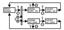
After select a menu signal, press OK. Then, using the UP and DOWN buttons to select the appropriate type of signal and enter the selection with the OK button. Entered message is the record of the name stored measured signal. Exit menu without saving the changes implemented by pressing the RESET button.
