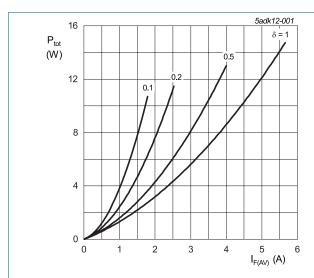
$$\begin{split} I_{F(AV)} &= I_{F(RMS)} \times \sqrt{\delta} \\ V_o &= 1.044 \text{ V; R}_s = 0.2758 \text{ }\Omega \end{split}$$
