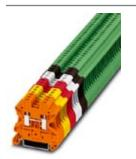
Feed-through terminal block, Connection method: Screw connection, Cross section: 0.14 mm<sup>2</sup> - 4 mm<sup>2</sup>, AWG: 26 - 12, Width: 5.2 mm, Color: orange, Mounting type: NS 35/7,5, NS 35/15
