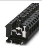
Fuse modular terminal block, Connection method: Screw connection, Cross section: 0.5 mm²- 16 mm², AWG: 20 - 6, Nominal current: 10 A, Nominal voltage: 400 V, Width: 12 mm, Fuse type: G / 6,3 x 32, Fuse type: Glass, Mounting type: NS 35/7,5, NS 35/15, NS 32, Color: black
