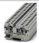
Feed-through terminal block, Connection method: Spring-cage connection, Cross section: 0.2 mm² - 10 mm², AWG: 24 - 8, Width: 8.2 mm, Color: blue, Mounting type: NS 35/7,5, NS 35/15
