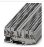
Disconnect terminal block, Connection type: Spring-cage connection, Cross section: 0.08 mm² - 4 mm², AWG: 28 - 12, Nominal current: 20 A, Nominal voltage: 400 V, Length: 84 mm, Width: 5.2 mm, Color: gray, Assembly: NS 35/7,5, NS 35/15
