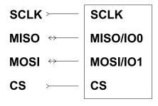
Figure 5. .SPI interface connection
