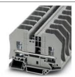
Bolt connection terminal block, Connection type: Bolt connection, Cross section: 2.5 mm² - 35 mm², AWG: 14 - 2, Nominal current: 125 A, Nominal voltage: 1000 V, Length: 84 mm, Width: 20.2 mm, Color: gray, Assembly: NS 35/7,5, NS 35/15
