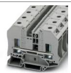
Bolt connection terminal block, Connection type: Bolt connection, Cross section: 2.5 mm² - 35 mm², AWG: 14 - 2, Nominal current: 125 A, Nominal voltage: 1000 V, Length: 84 mm, Width: 20.3 mm, Color: gray, Assembly: NS 35/7,5, NS 35/15
