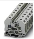
Bolt connection terminal block, Connection type: Bolt connection, Cross section: 0.1 mm² - 6 mm², AWG: 26 - 10, Nominal current: 41 A, Nominal voltage: 1000 V, Length: 66 mm, Width: 16.3 mm, Color: gray, Assembly: NS 35/7,5, NS 35/15
