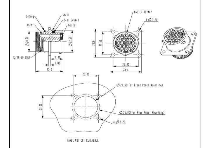
**TECHNICAL DATA** TEMPERATURE RANGE: -40°C to + 105°C PROTECTION: IP67 in mated condition and in combination with sealed backshell **VOLTAGE RATING** 150V HOUSING BODY: Zinc Alloy, Nickel Plated COUPLING NUT: Glass-filled Thermoplastic UL94-V0 INSERT: SEAL: NBR **CURRENT:** 5A with Stamped and Formed Contact / 7.5A with Machined Contact **CONTACT SIZE:** 20Awg **APPROVALS:** UL ECBT2
