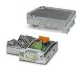
D-SUB plug, 9-pos., pin, axial version with two cable entries, below 35°, bus system: PROFIBUS DP up to 12 Mbps, termination resistor can be switched on via slide switch, pin assignment: 3, 5, 6, 8; spring-cage connection terminal blocks
