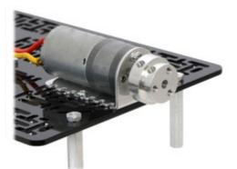
The machined piece of the 4 mm scooter wheel adapter mounted to the output shaft of a 25D mm gearmotor.
