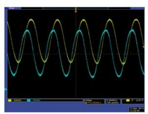
5V encoder version, motor approx. 30k RPM: 5-tooth wheel way too far from sensors.
