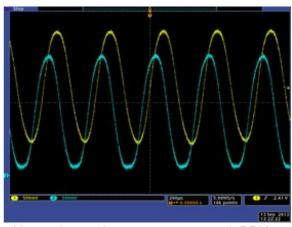
5V encoder version, motor approx. 30k RPM: 5-tooth wheel slightly too far from sensors.
