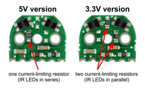
The 5 V version with LEDs in series draws approximately 12 mA; the 3.3 V version with LEDs in parallel draws approximately 24 mA.
