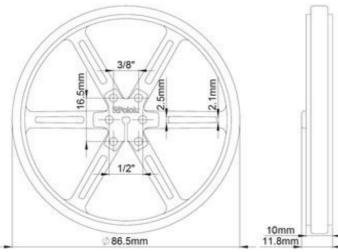
Mechanical drawing of Pololu wheel 90×10mm without tire.
