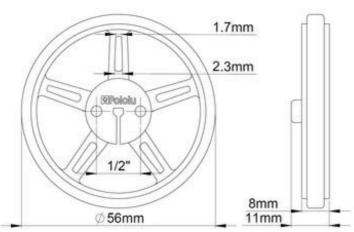
Mechanical drawing of Pololu wheel 60×8mm without tire.
