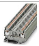
Disconnect terminal block, Connection type: Push-in connection, Cross section: 0.14 mm² - 4 mm², AWG: 26 - 12, Nominal current: 20 A, Nominal voltage: 400 V, Length: 62 mm, Width: 5.2 mm, Color: gray, Assembly: NS 35/7,5, NS 35/15
