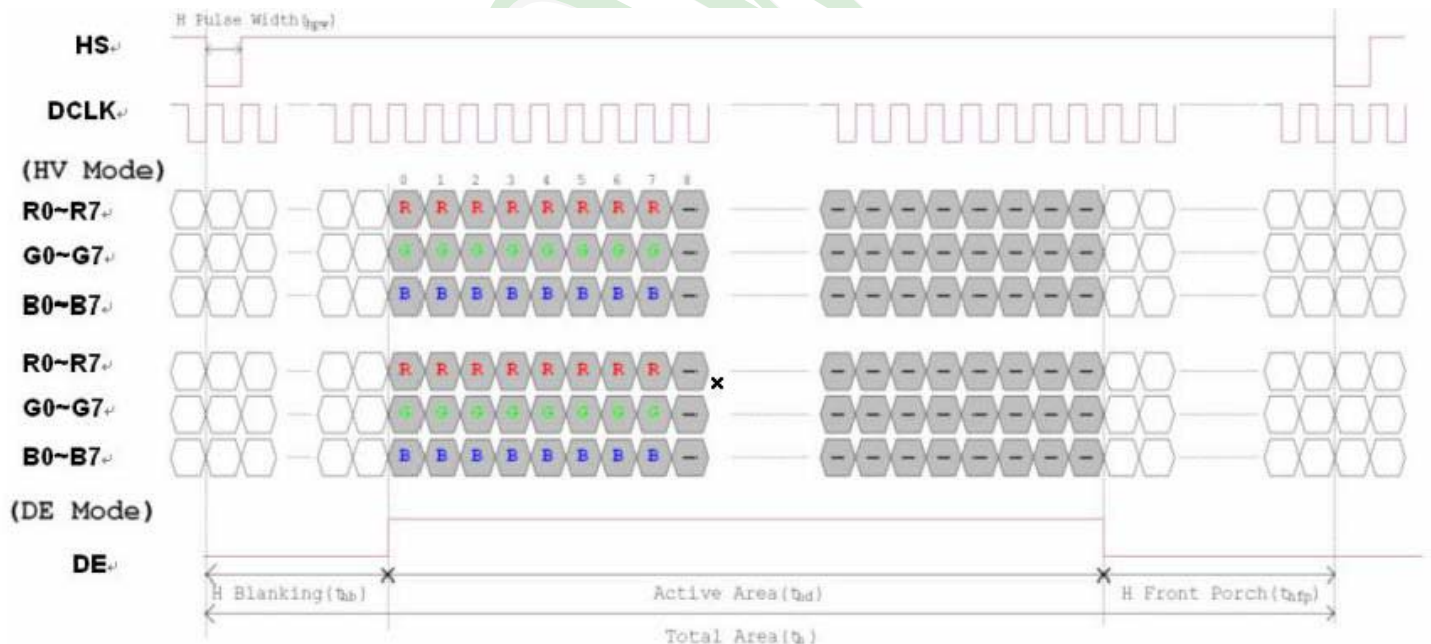
Horizontal input timing diagram
