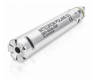
**OXY-DIOS-DSP** is a high quality process, dissolved oxygen sensor applied in sewage, potable and industrial water. Our sensor assures fast measurement response and minimal drift. In typical applying conditions it requires calibration once a year, and measuring windows replacement every two years. By using measurement method, our device does not need electrolytes and replaceable membrane.
