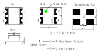
Notes: 1. All dimensions are in millimeters; 2. Tolerance is  $\pm$  0.10 mm unless otherwise noted.
