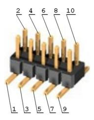
Note that pin 7 of SWD connector is cut off.
