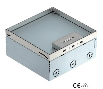
Square floor box for use in dry-cleaned cavity and screed floors for indoor use. Installation housing with pre-marked insertion openings for pipelines (M25). Cover adjustable to top edge of floor covering using four height-adjustment supports. 15 mm floor covering recess in the hinged cover. The minimum installation depth is 95 mm, the height-adjustment range  $\pm$  30 mm.
