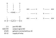
RS-485 port is not galvanically isolated from power supply module.
