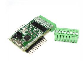
The module is used for remote control, using any IR remote control that utilizes the popular RC5 code. A small size, built-in 3 channels and routed pins from the microcontroller give you the chance to extend the set with additional functions.
