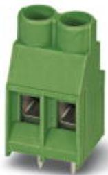
PCB terminal block, Nominal current: 32 A, Nom. voltage: 630 V, Pitch: 6.35 mm, Number of positions: 2, Connection method: Screw connection with tension sleeve, Mounting: Wave soldering, Conductor/PCB connection direction: 0 °, Color: green, The article can be aligned to create different nos. of positions!
