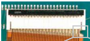
Incomplete FPC insertion
