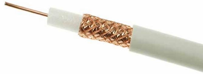
High-frequency coaxial cable (W), with an internal single core conductor (D), with polyethylene foam (p) insulation, with armoring comprising copper wire braiding (ek), in PVC sheathing (Y).
