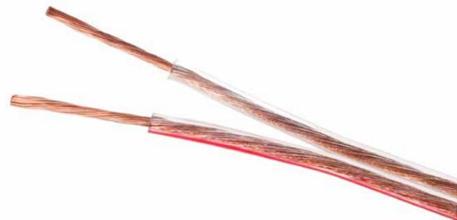
Flat PA and speaker cables, with a multi-strand conductor and transparent PVC insulation. One of the conductors is marked red. Telecommunication cable (T), WITH multi-strand, copper conductors (L), WITH shared PVC insulation (Y), flat (p).
