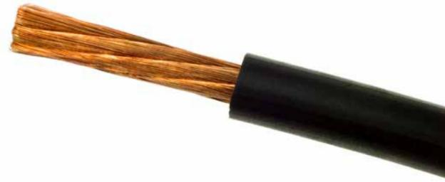
Rubber-sheathed cables with normal-flexibility conductors. The cables are manufactured in accordance with a harmonized standard (H), intended to support rated voltage of 100/100V (05), with chloroprene rubber sheathing (N2), with normal-flexibility conductors (D). Cables resistant to oil, gasoline, light, ozone, oxygen and protective gas.
