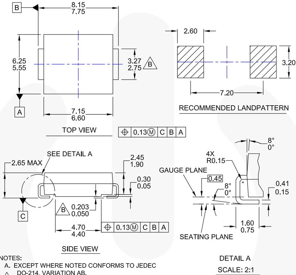
Figure 6. 2-LEAD, SMC, JEDEC DO-214, VARIATION AB (ACTIVE)
