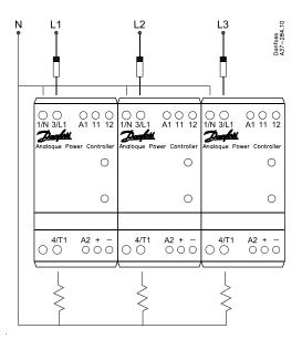
Max. load at: 230 V 3 x ACI 30-1 20.7 kW 3 x ACI 50-1 34.5 kW Three phase with single-phase contactor ECI-1 as slave
