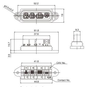
Based on the above diagram, the number of positions for each mating port is as follows from left to right: 3, 4, 6 and 2pos.
