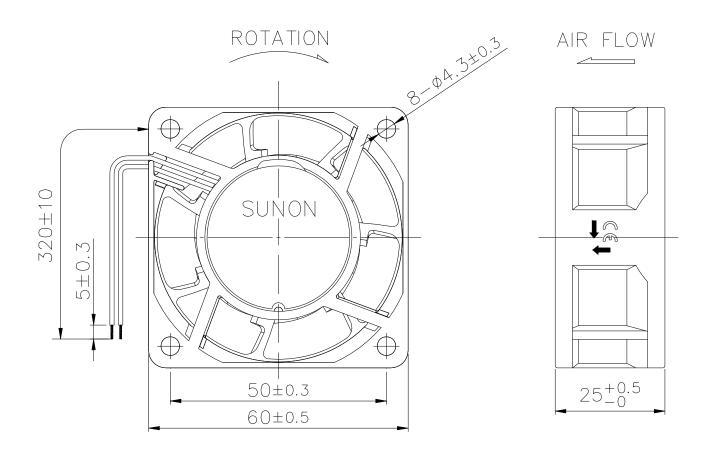
NOTE: 1.LEAD WIRE:UL3266 #24AWG GRAY 2.FRAME TYPE:FLANGE
