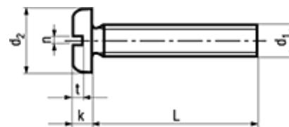
**BN 1404****Slotted pan head machine screws**
