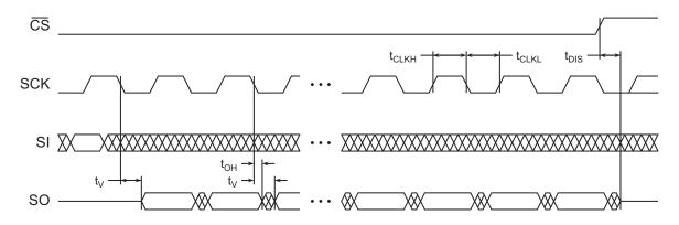
Figure 15-3. WP Timing for Write Status Register Byte 1 Command When SPRL = 1
