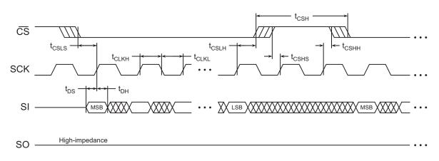
Figure 15-2. Serial Output Timing
