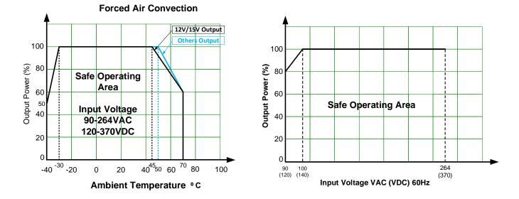
Note: With an AC input voltage between 90-100VAC and a DC input between 120-140VDC the output power must be derated as per the temperature derating curves.
