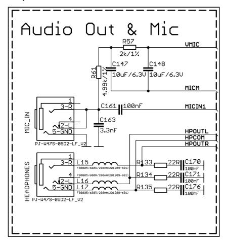
Standard MIC\_IN jack is mounted for audio input to the board. Note that it is a single channel MIC\_IN. The MIC\_IN is a mono input.
