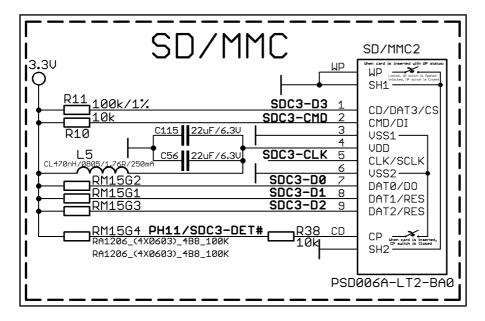
The SD/MMC2 slot is located on the back of the PCB and works with the "larger" SD and MMC cards. The connector was placed by a popular demand.
