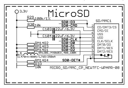
SD/MMC1 slot is the "smaller" microSD card slot, located on the top of the board.
