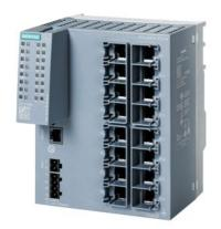
SCALANCE XC216 manageable Layer 2 IE switch; IEC 62443-4-2 certified; 16X 10/100 Mbit/s RJ45 ports; 1x console port, diagnostics LED; redundant power supply; temperature range -40 °C to +70 °C; assembly: DIN rail/S7 mounting rail/wall Office redundancy functions features (RSTP, VLAN,...); PROFINET IO device; Ethernet/IP-compliant; C-plug slot;
