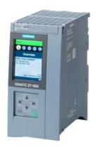
SIMATIC S7-1500, CPU 1516-3 PN/DP, central processing unit with 2 MB work memory for program and 7.5 MB for data 1st interface: PROFINET IRT with 2-port switch, 2nd interface: PROFINET RT, 3rd interface: PROFIBUS, 6 ns bit performance, SIMATIC Memory Card required \*\*\* approvals and certificates according to entry 109817466 at support.industry.siemens.com to be considered! \*\*\*
