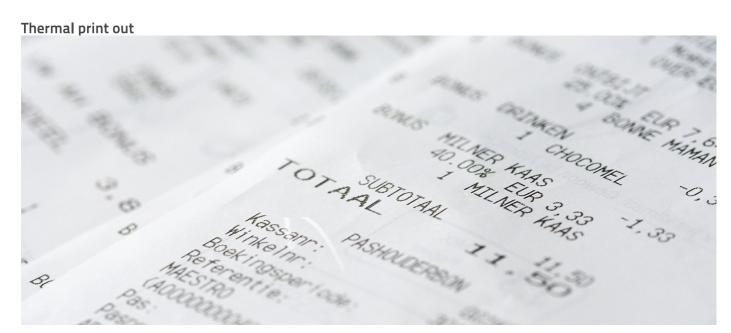
Thanks to the direct printing method, which is highly sensitive to temperature, the device doesn't require ink or toner. Printouts are made immediately by heating the paper placed inside the printer.
