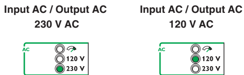
Figure 26 LED indicators in mains or battery mode
