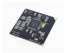
The module has the same form factor of FlyportPRO Wi-Fi and FlyportPRO GPRS and the pinout is compatible.
